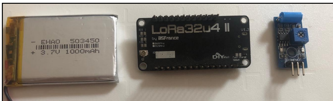
Figure 16 – LoRa end-device used by MonitBee (testing app)with tilt sensor and 1000 mAh battery.
