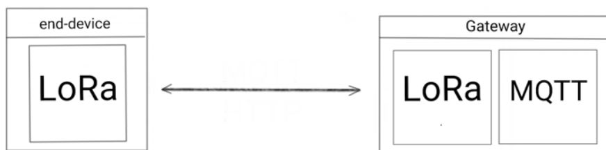
Figure 15 – LoRa communication between end-device and gateway.
