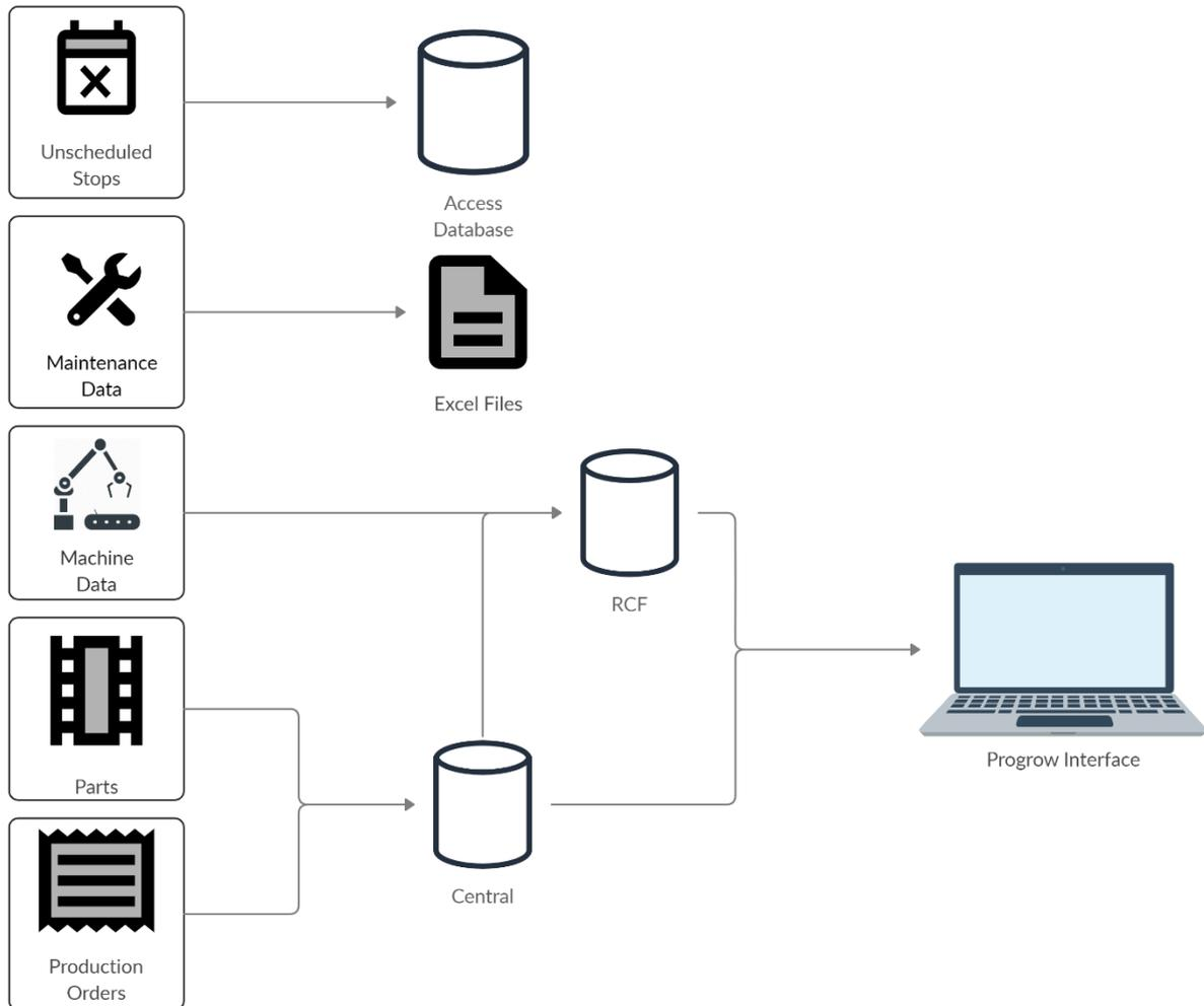
*Figure 17 - Data flow of HFA production*
