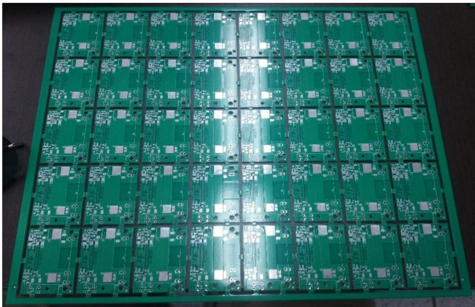
*Figure 19 - Example of a finished Set of 40 PCB's*
