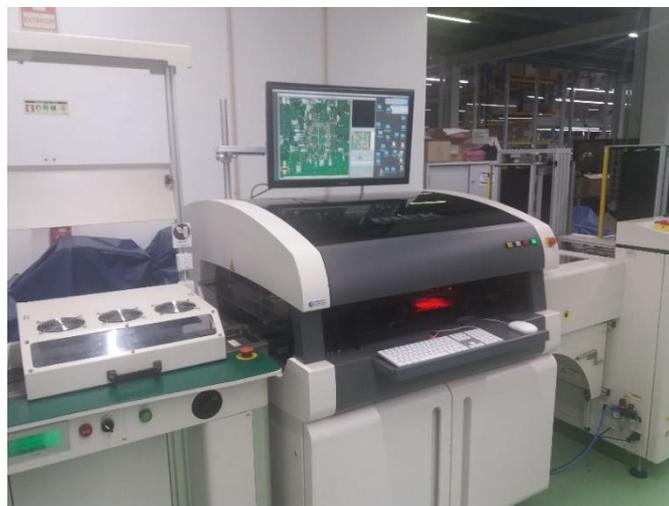
*Figure 16 - Production line six AOI*
