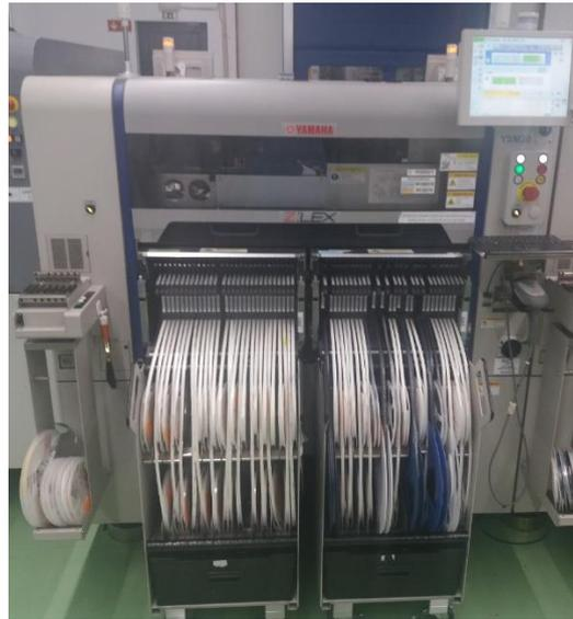
*Figure 14 - Production Line six Pick and Place*
