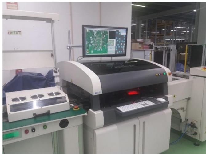
*Figure 16 - Production line six AOI*
