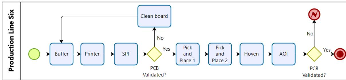
*Figure 18 - Production line six layout*
