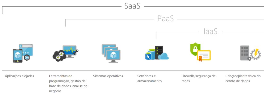
Figura 6 – Componentes dos modelos Software as a service, Platform as a service e Infrastructure as a Service (Fonte: Microsoft Azure)
