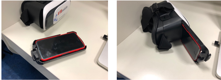
Figure 11 - Insert device onto VR Googles
