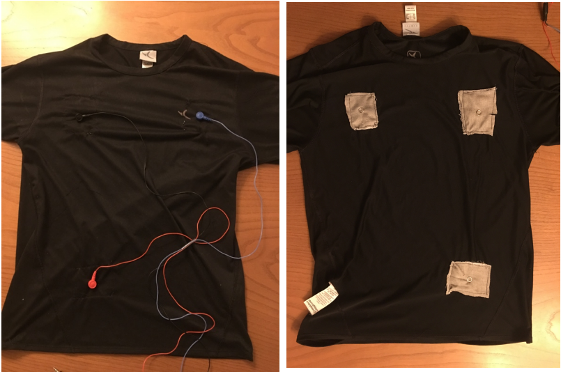
Figure 26 - E-Textile ECG t-shirt
