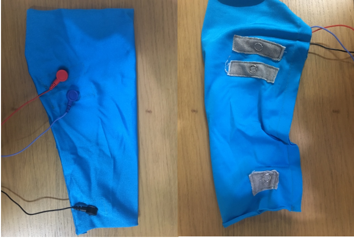
Figure 25 - E-Textile EMG shinguard
