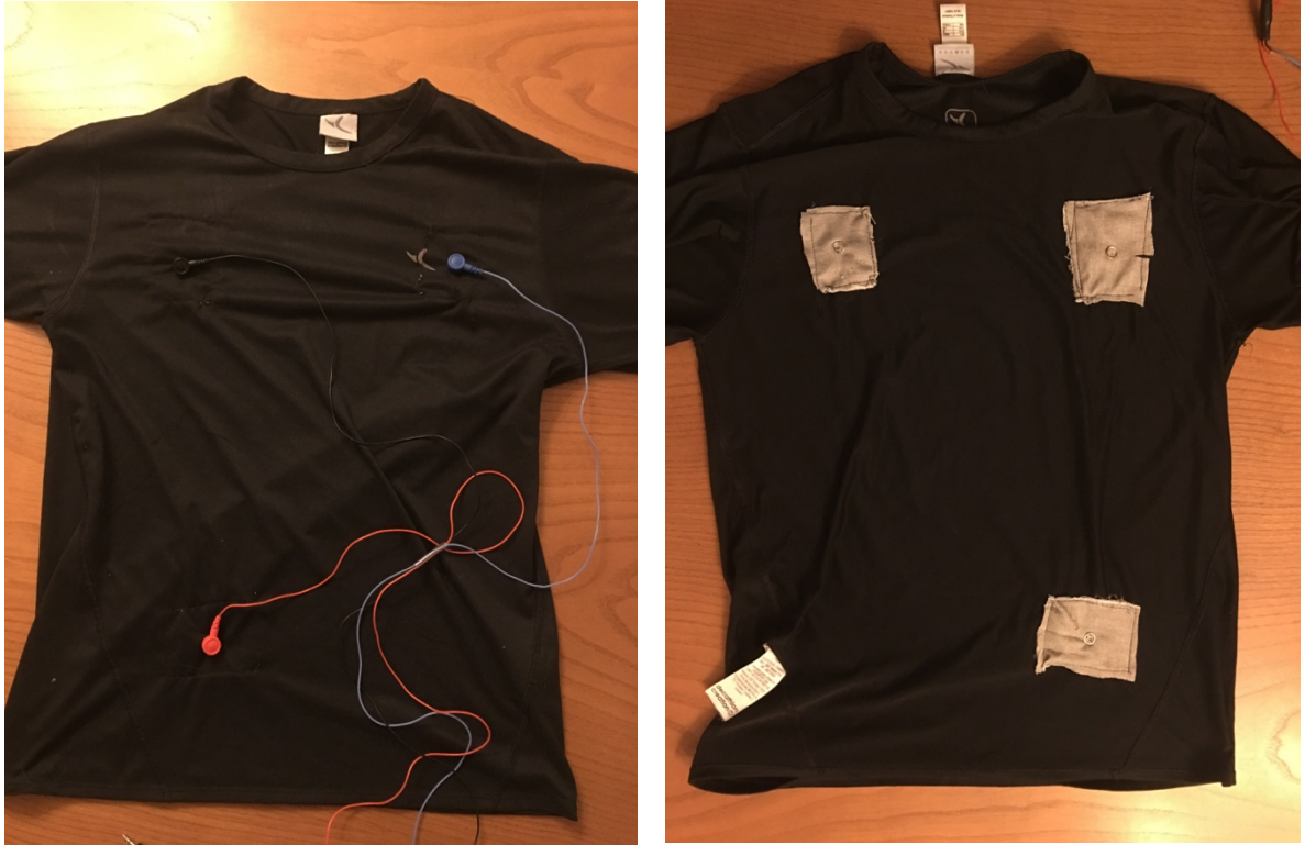
Figure 5.10 - E-textile electrodes t-shirt
