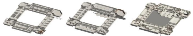
Fig. 1. 3D section views of the BIM model of ISCTE-IUL’s Building 1 – Sedas Nunes
