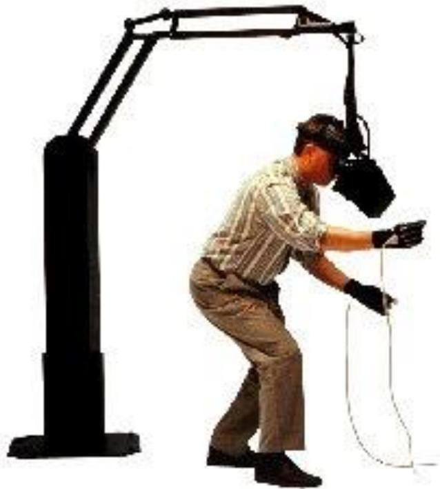
*Figura 13 BOOM (Binocular Omni Orientation Monitor). Retirado de <https://realitevirtuelleprojet.wordpress.com/histoire/dernieres-inventions/>*
