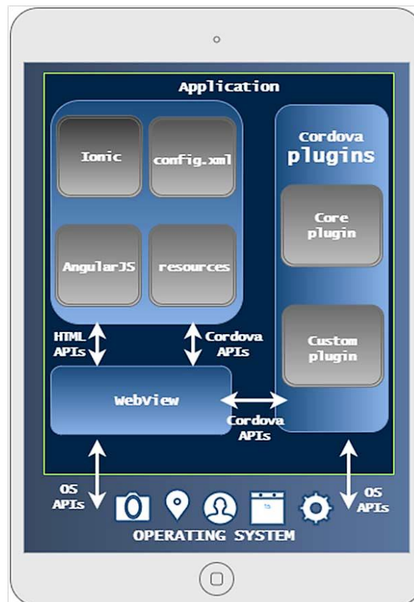
Figure 17 - Hybrid applications architecture and usage of Apache Cordova tools (Bosniac et al., 2017)
