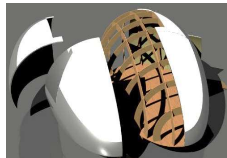
Figure 7. Final module's 3D modulation: Extruded aluminium plaques
