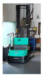
Figure 4 - Electric powered rider straddle Truck
