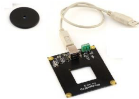
Fig. 4. LF RFID reader embedded in the box and LF tags embedded in the red and green color cubs for cubs' identification.
