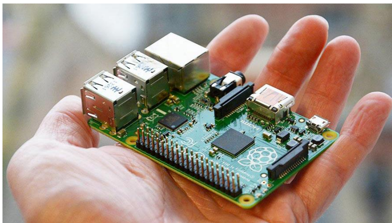
Figura 3. Microprocessador- Raspberry Pi
