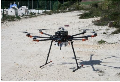
Figure 2- 12. Octocopter (drone) with TSMA attached (under it)
