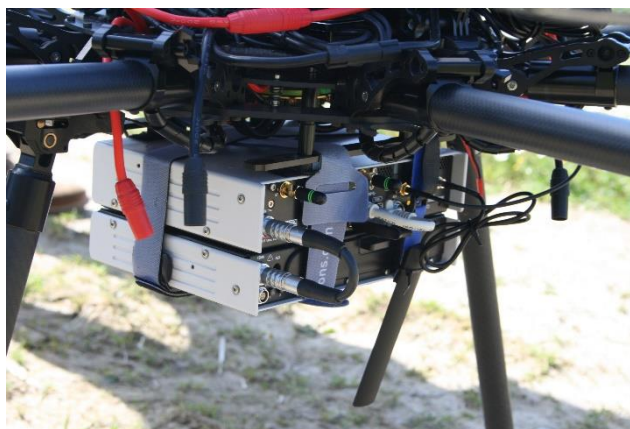
Figure 4-5. Equipment attached below the drone with velcro tape
