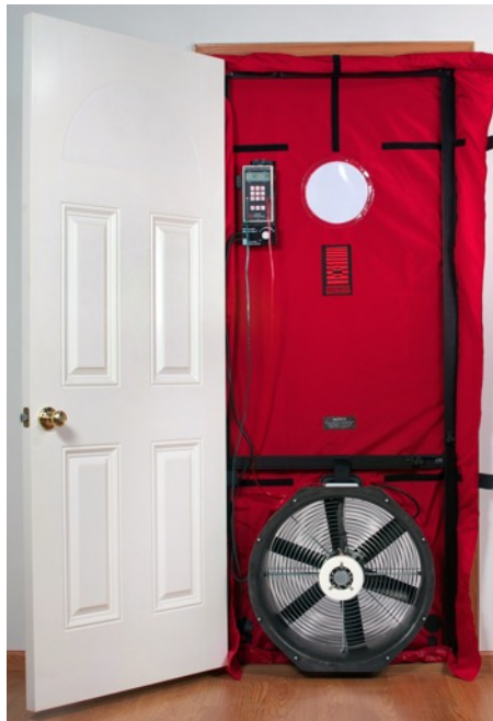
Figure 5: Blower Door Test
