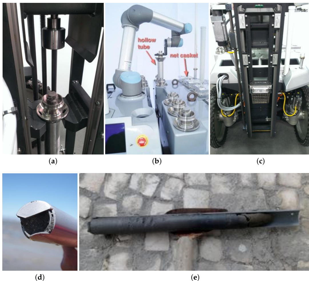
Figure 5. The drilling and dredging tools. (a) A hollow tube being attached to the drilling tool; (b) the robotic arm grasping a hollow tube to insert it into the drilling tool; (c) a dredger being pushed downwards by the drilling tool; (d) the hollow tube's tip designed to prevent the core from slipping during extraction; (e) a sediment sample laid on the PVC half-tube after extraction.
