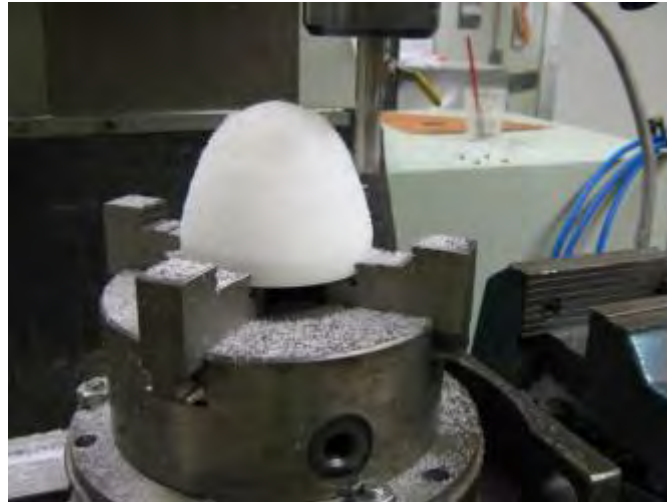
Figure 28 - Lens fabrication by CNC milling machine technique.
