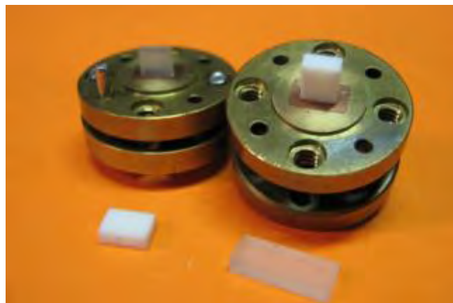
Figure 26 - Example of waveguide short-circuited sample-holder for V-band and a few dielectric samples.
