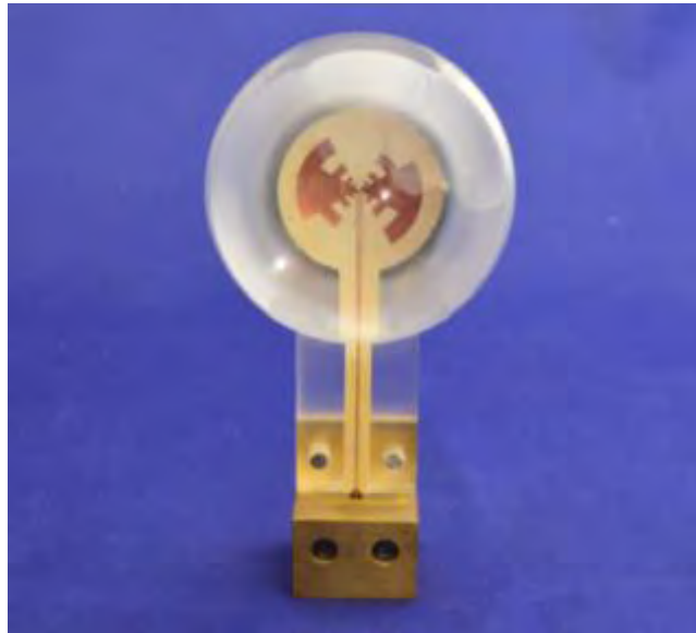
Figure 30 - Integrated lens antenna fed by a planar self-complementary log-periodic feed.
