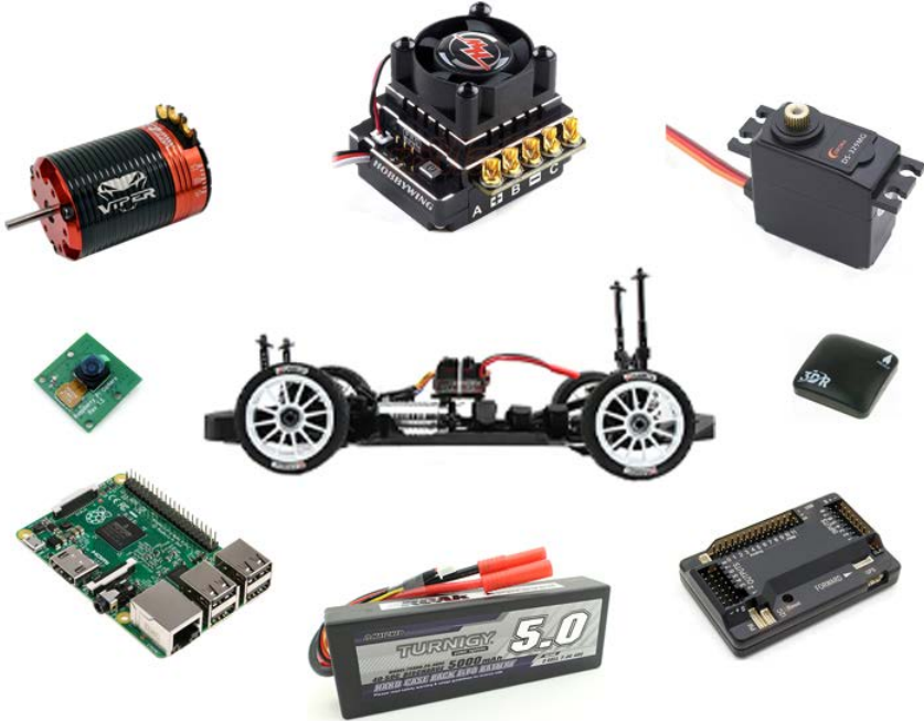
Figure 3.1 – UGV composition and all on-board components.
