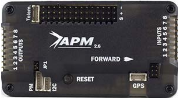
Figure 4.2 – APM 2.6 with enclosure. Source: [86].
