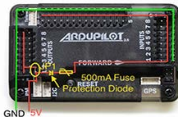
Figure 4.5 – APM 2.6 dual positive rails. Source: [96].
