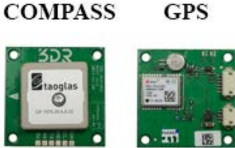
Figure 4.1 - uBlox LEA-6H GPS module with on-board compass.
