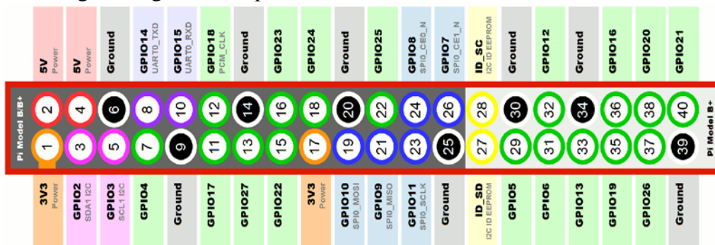
Figure 4.9 – RPI2 GPIO header. Source: [114].
